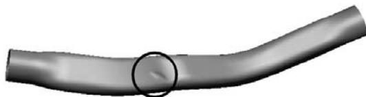
Fig. 13 Irreversible deflection because of a too large a tube diameter ; with shell element
