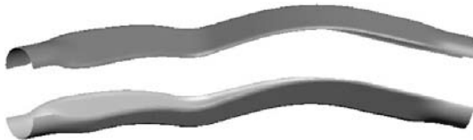
Fig. 6 Upper and lower part of the die
