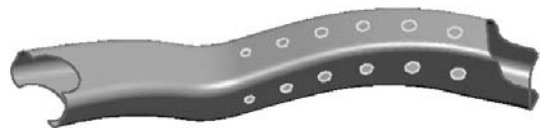
Fig. 2 Picture of the axial component with the tube start, the tube end and the indicated filled holes
